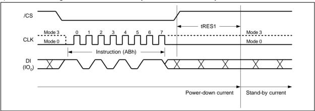
Figure 38a. Release Power-down Instruction (SPI Mode)
