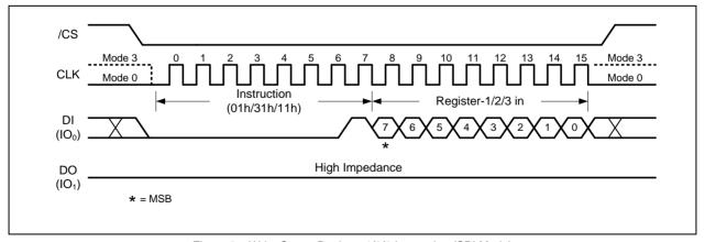
Figure 9a. Write Status Register-1/2/3 Instruction (SPI Mode)
