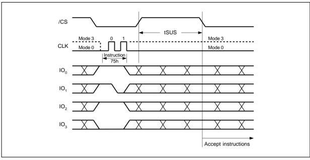
Figure 35b. Erase/Program Suspend Instruction (QPI Mode)
