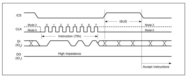
Figure 35a. Erase/Program Suspend Instruction (SPI Mode)
