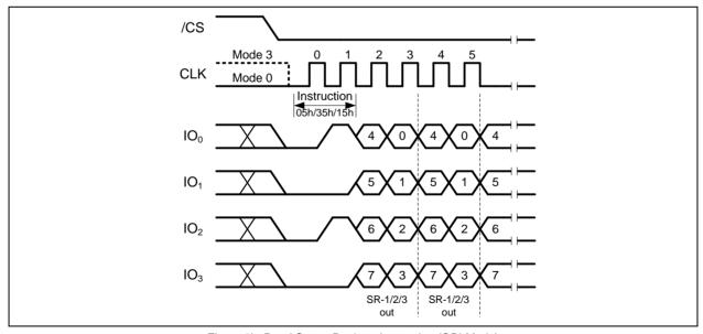
Figure 8b. Read Status Register Instruction (QPI Mode)
