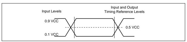
Figure 59. AC Measurement I/O Waveform
