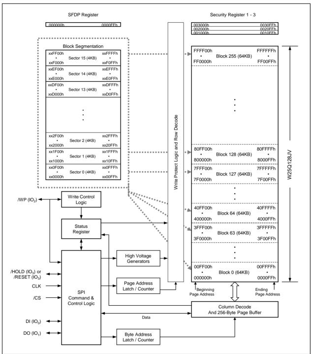
Figure 2. W25Q128JV Serial Flash Memory Block Diagram
