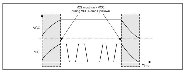
Figure 58b. Power-up, Power-Down Requirement
