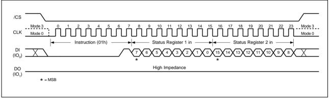
Figure 9c. Write Status Register-1/2 Instruction (SPI Mode)
